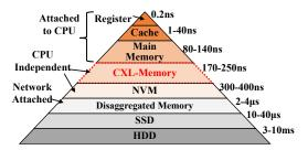
Figure 2: Latency characteristics of memory technologies.
