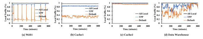
Figure 14: Fast cold page demotion and effective hot page promotion allow TPP to serve most of the traffics from the local node.
